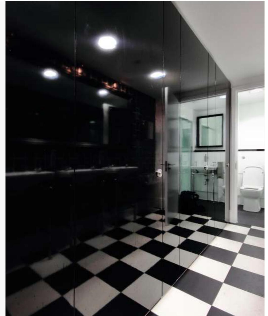
Decra Burj Gloss true full height cubicle system with black gloss laminate faced doors and pilasters
